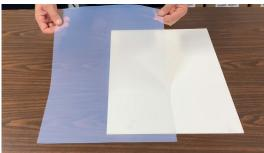
2. Prepare one sheet of Screenmate<sup>TM</sup> Film and the ScreenMate<sup>TM</sup> Film Guide. The ScreenMate<sup>TM</sup> Film must have the printing side facing up.
