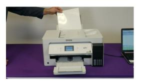
6. Load the ScreenMate™ together with the Film Guide with the corners first and the printing side facing up.
