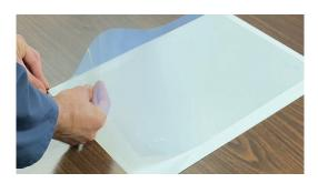
4. ScreenMate™ Film needs to be aligned with the edge when it is inserted into the Film Guide corner.
