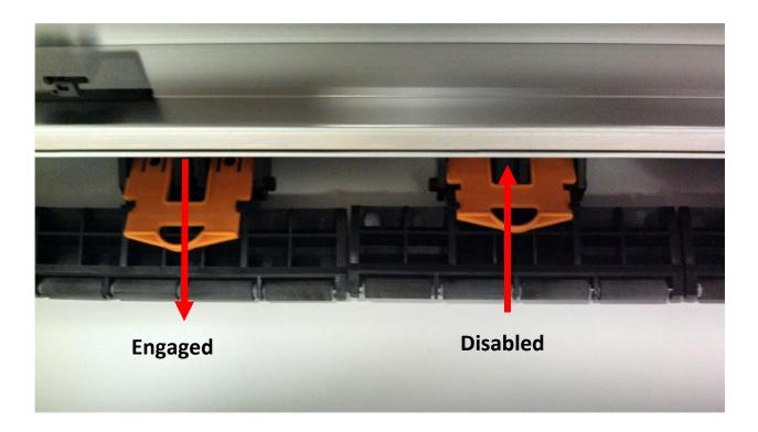
If the papers start to cockle causing head strikes, it is recommended to cancel/disable the first 2-4 rollers on both edges of the media, depending on media width. Keep as many rollers as needed engaged in the center of the media to ensure proper feeding.
