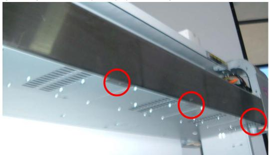
Start by removing the five screws that hold the front plate in. Three of these screws are circled in red on the above image.
