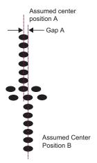
4. If any abnormal conditions are found, identify the difference between the CW printing position and the CCW printing position and enter the difference as the repeatability adjustment parameter.
