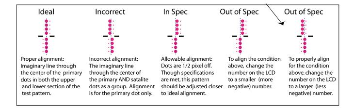
As with the Uni-D (CW) alignments, 1 dot of movement equals 9 increments on the display.
