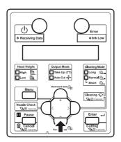
• Displays the remaining length of data currently being printed.
