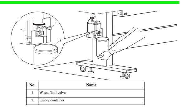
4. After pouring the waste fluid to the empty container, close the waste fluid valve securely.
