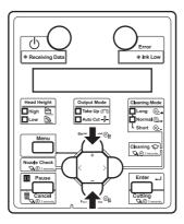
5. To save the changed setting, press the [Enter] key on Operation panel.
