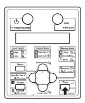
• When head cleaning is complete, "Wash retry? No" is displayed on Operation panel.
