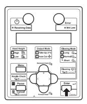
• When head cleaning is complete, "Wash retry? No" is displayed on Operation panel.
