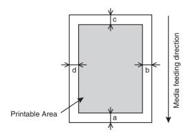
a=5mm \*1 b=5mm to 25mm c=5mm d=5mm to 25mm
